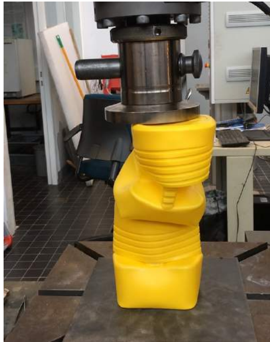
Figure 5.17: stacked drill containers I test 4
